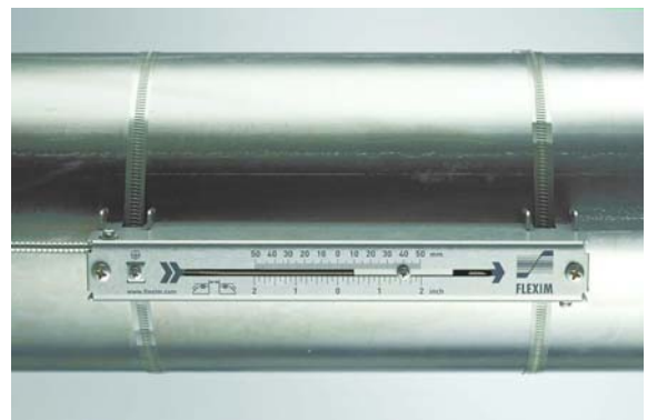
Measurement with transducers mounted by Variofix L
