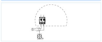
Connection of the voltage supply in electronics housing
