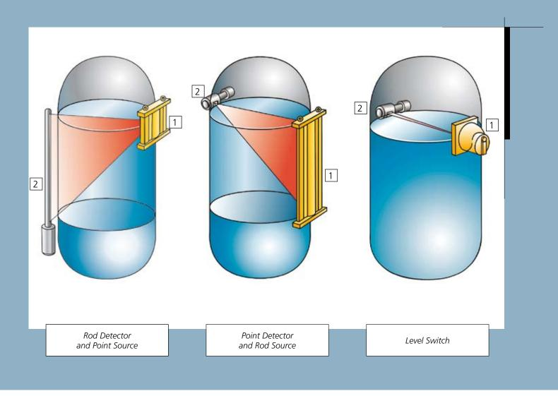
Figures above show schematic layouts of typical measuring arrangements, comprising the source 1 mounted on the outside of the container, and the Uni-Probe 2. Source and Uni-Probe have to form a radiation field correspond-
