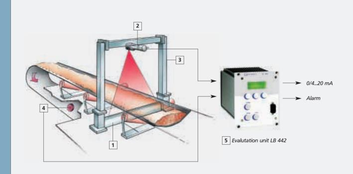
How does the LB 442 operate? The rod-shaped radiation source is specially designed for the application as regards loading, material and the conveyor system. The radiation source is installed in a lockable shielding which is mounted under the conveyor. The scintillation counter is installed on top of the conveyor and is in line with the radiation source. The intensity of the radiation received by the scintillation counter is a measure of the loading on the conveyor system.
