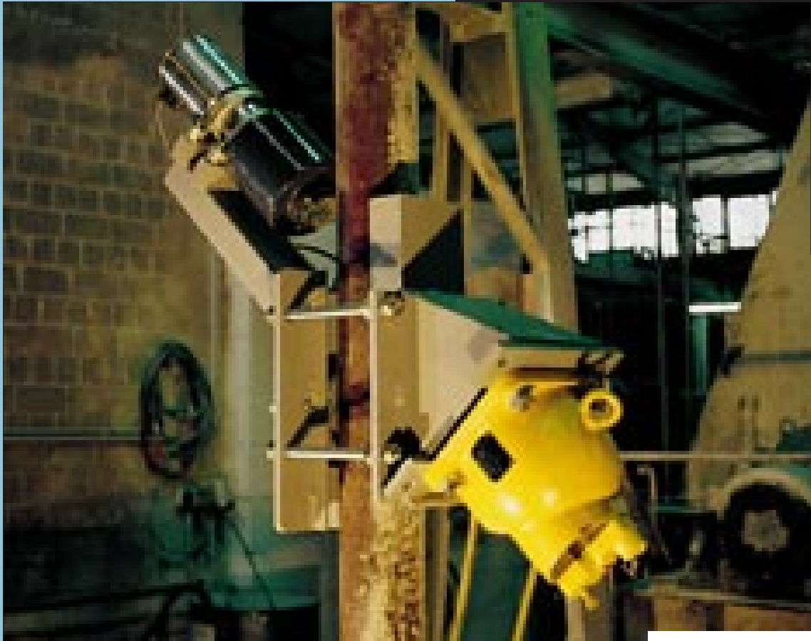
ARRANGEMENT FOR 45° IRRADIATION
