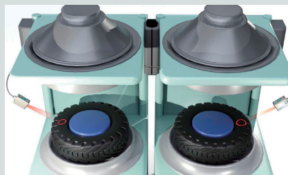
Controlling heating time in tire vulcanization processes
