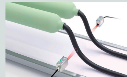
Measuring temperature in rubber extrusion processes
