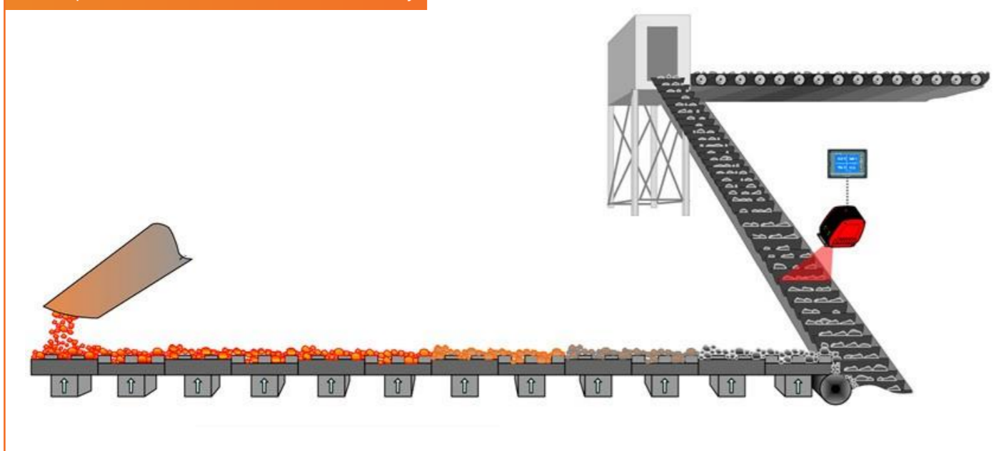
A HotSpotIR sensor installed to scan the conveyo
