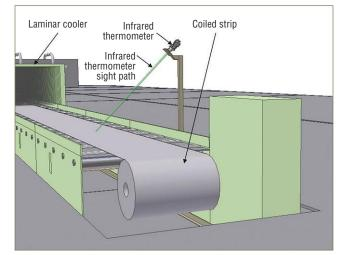
Fig. 1. A single-point pyrometer measuring the centerline temperature of a hot strip.
