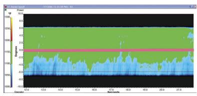
Fig. 8. Cold operator side caused by improper cooling. The red stripe shows how a single-point pyrometer would miss the problem.
