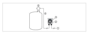
Connection of the VEGADIS 82 to the sensor, adjustment via the display and adjustment module
