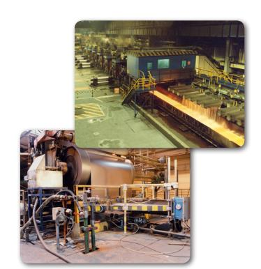
Photos (Top to bottom): Hot Strip Mill - Cooling Section, Galvanising line
