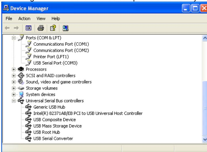
6. The USB-RS485 Modbus converter will now operate on COM3 (in this example).
