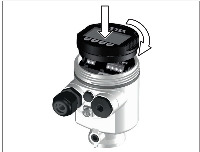
Fig. 36: Insertion of the display and adjustment module with single chamber housing into the electronics compartment
