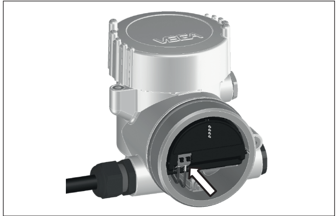
Fig. 19: Connection steps 5 and 6 - Double chamber housing
